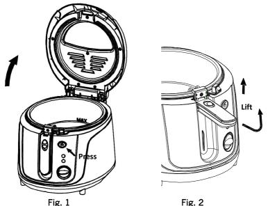
2. Place the fryer on a stable, flat, heat resistant surface and away from flammable materials and surfaces that may be damaged by steam. Check that the plug will reach a socket and that it can be accessed without reaching over the fryer.
